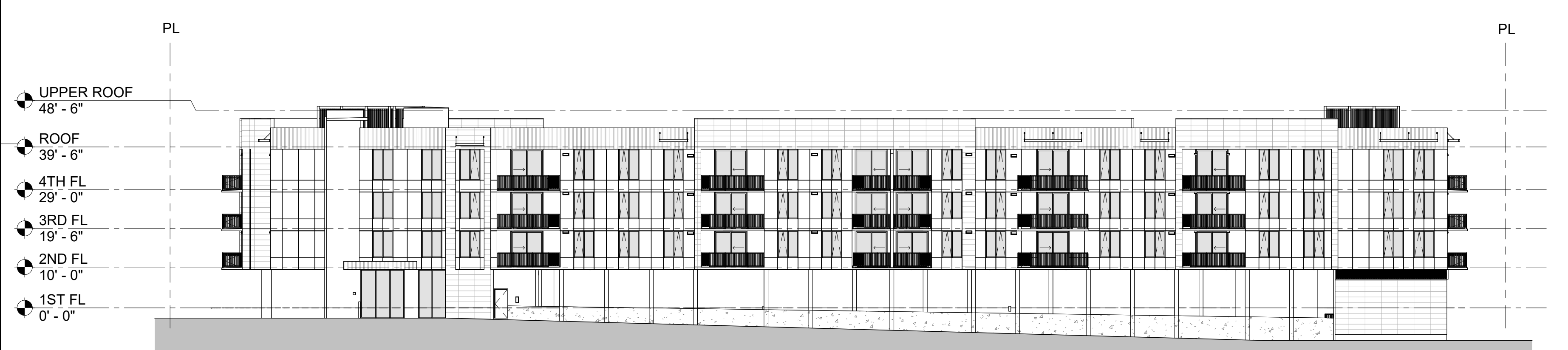
A1 BUILDING B - WEST ELEVATION 1" = 20'-0" CPR-3.01
